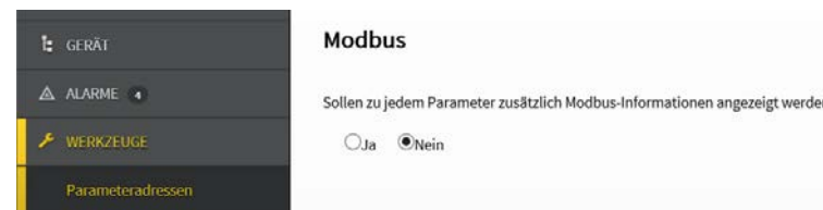
Activation of Modbus register display
